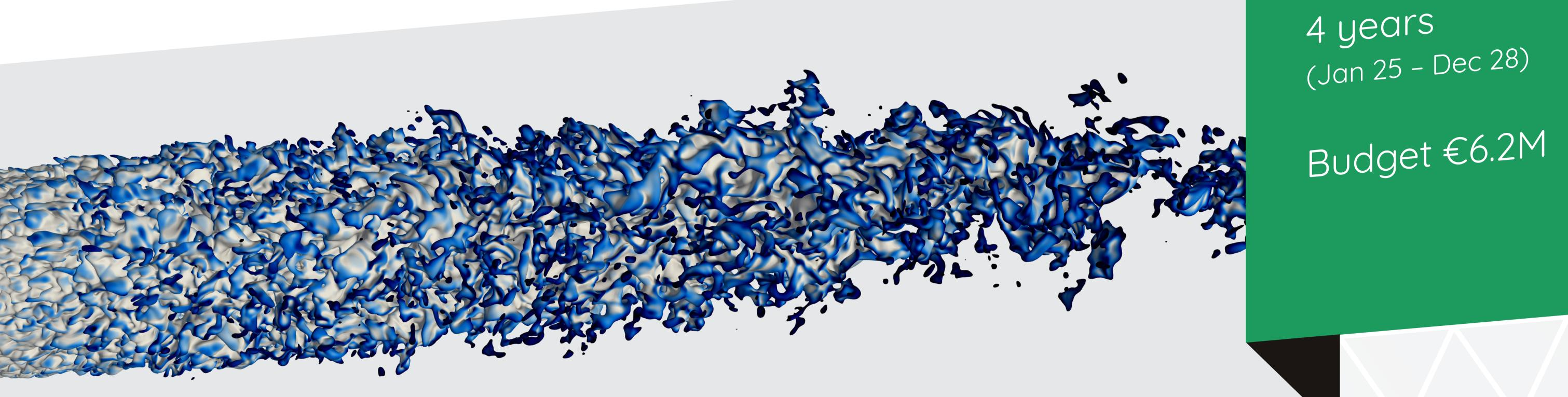
Turbulent premixed hydrogen/air flame at gas turbine conditions (Image courtesy of RWTH Aachen)
